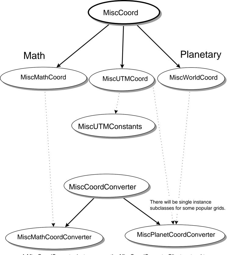
A MiscCoordConverter instance uses the MiscCoordConverterClient protocol to communicate with MiscCoord classes that it is able to convert between. A MiscCoord class initiates the request to the MiscCoordConverter that is its delegate. There is only one instance ever created of a given converter, meaning that converters are not reentrant at present.
