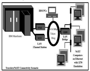
This scenario will allow the NeXT Computer to achieve host access through Token Ring, by using Conextion's SCSI to Token Ring hardware device. 3270 Vision software will again be used to give the NeXT full screen 3270 emulation with up to five concurrent host sessions. The NeXT Computers will be able to communicate with other IBM PC and RT computers connected to the Token Ring. The cost of this solution would be about \$1500 for Conextion's hardware and software.
