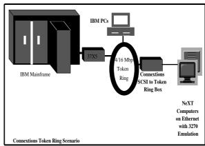
\* Ethernet to Token Ring Bridge with Transparent Bridging and Source Routing.
