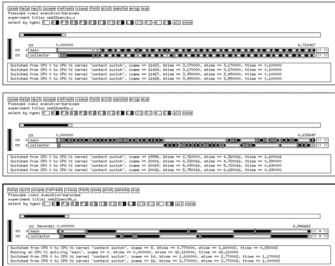
Figure 5: The Execution of Two Threads on Three Kernels: XF29, CS5a, X96
