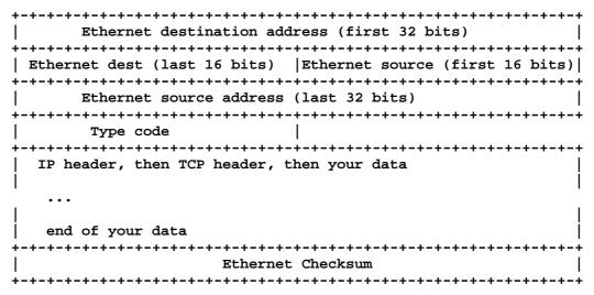
If we represent the Ethernet header with "E", and the Ethernet checksum with "C", your file now looks like this: EIT....C EIT....C EIT....C EIT....C
