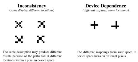
In the **ControlPoint** application, an array is created at initialization time that contains 1000 point locations. These locations are selected to randomly fall at different locations within a pixel. Since the control points are 5 points or less across, some care must be taken to ensure that the points are displayed consistently.
