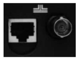
Regardless of the Ethernet cable option you choose, adding a NeXT computer to the network is a simple task: simply connect the computer to the network and turn it on. NeXTstep $^{\text{TM}}$  automatically senses which type of Ethernet wiring you have used and correctly configures itself. It's that easy.
