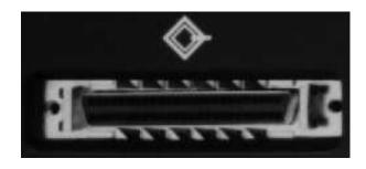
NeXT computers implement the SCSI-1 protocol using a SCSI-2 connector. When the SCSI-2 protocol is fully defined, NeXT will implement and support it. Until then, NeXT will be compatible with all existing SCSI-1 devices. NeXT also provides cables connecting SCSI-1 and SCSI-2 connectors.
